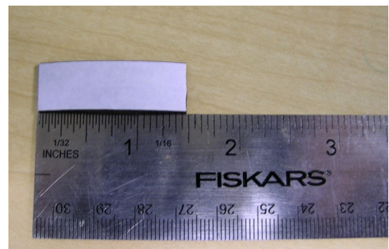
Figure 2.14 Recommended Length of 0.5 Inch for Magnetic Strip
